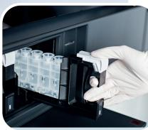
The STRATEC Reagent Rack and Bay system is a flexible and smart module for reagent loading and storage in fully automated analyzers. Autonomous Reagent Racks are equipped with a flexible agitation functionality and a read/write RFID technology for reliable reagent identification and management.
