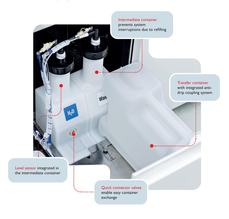
Intermediate containers with level detection and quick connector systems enable refilling of system liquids without interruptions and spillage. There is no need to switch tubes or level detection from one container to another.
